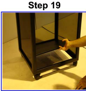
Step 19 Position and set in place bottom shelf into pre-assembled bottom frame.
